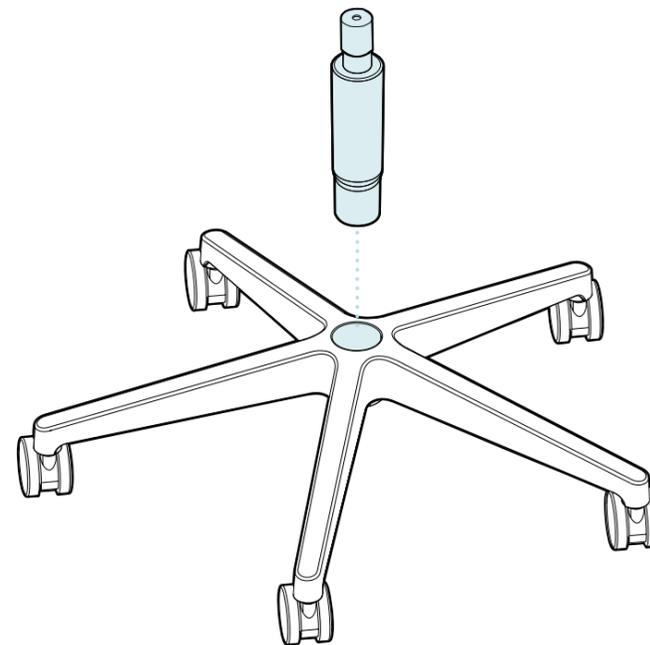
Place the piston into the center of the base with the smaller end pointed up.
