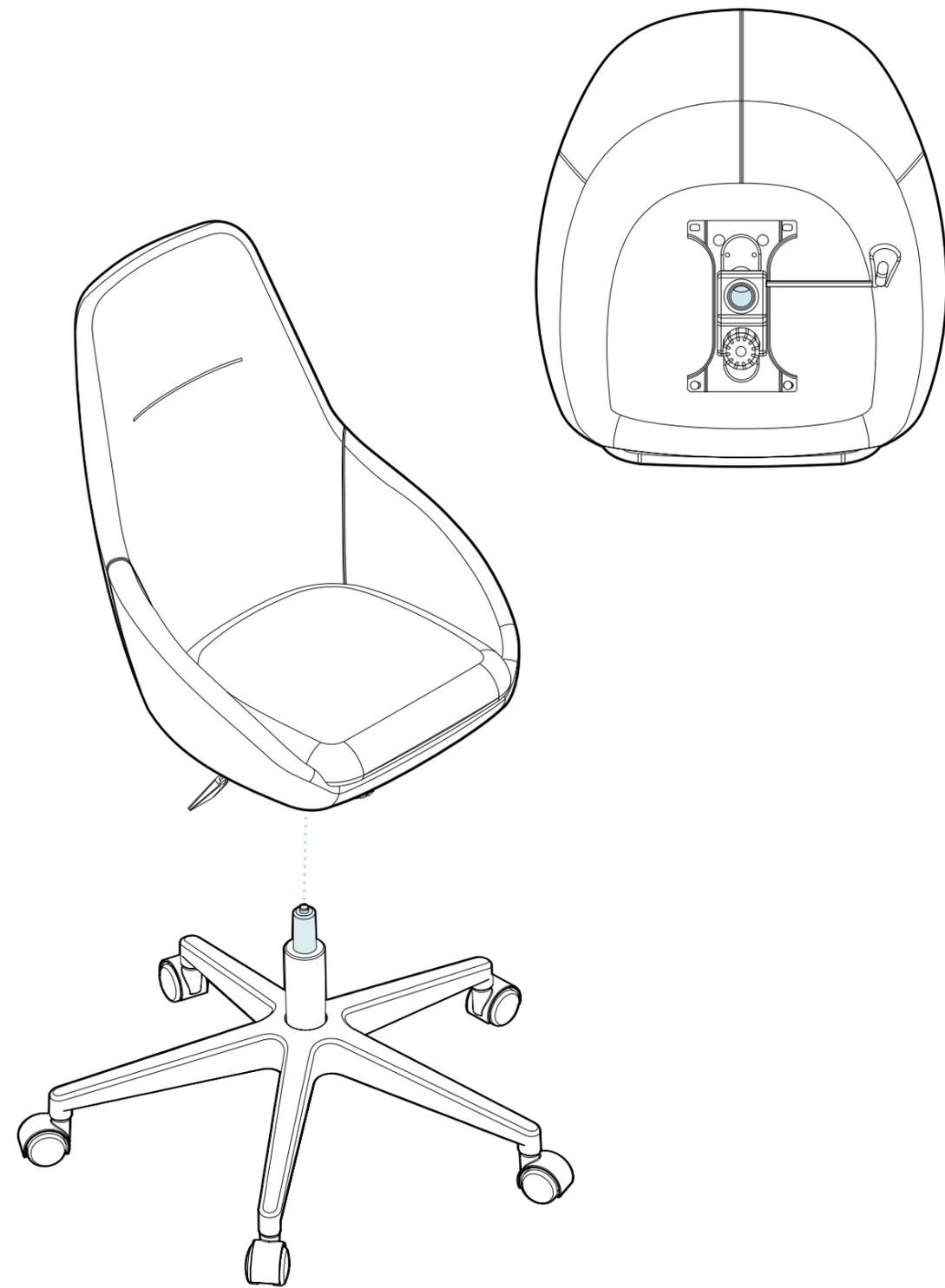
With assistance, take the chair seat and place the highlighted section of the mechanism onto the highlighted section of the piston.
